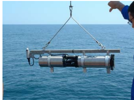
Fig.3 Fast Rate Repetition Fluorimeter (photo by G.Shapiro)
