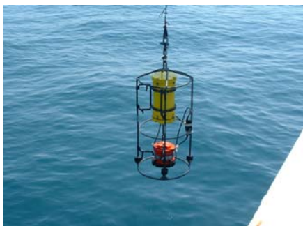
Fig2. Lowered Acoustic Doppler Current Profiler (photo by G.Shapiro)
