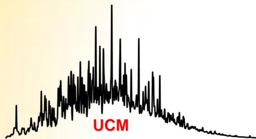
**Figure 1.** GC-MS mass chromatogram of a soil contaminated with aviation fuel oil.
