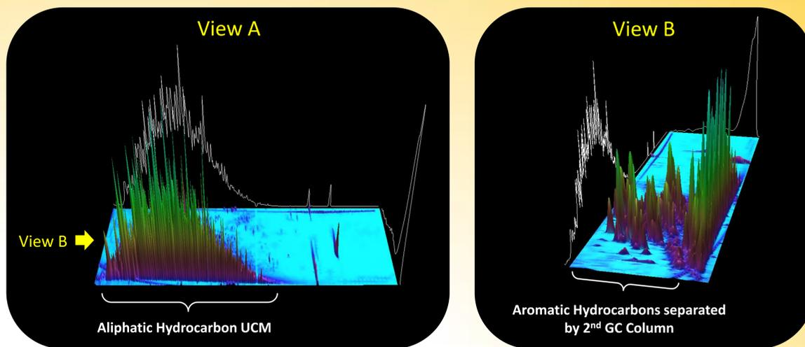
**Figure 2.** GCxGC-ToF-MS Total ion mass (TIC) chromatogram of a soil contaminated by aviation fuel oil.
