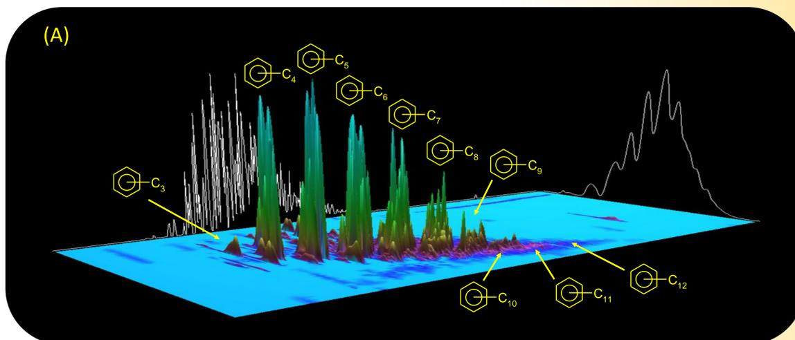
**Figure 3. (A)** Example extracted ion mass chromatogram ( $m/z$  133+119+105) showing the chromatographic separation of C<sub>3</sub> to C<sub>12</sub> branched alkyl benzene isomers. **(B)** Chromatographic separation of individual C<sub>11</sub> ( $m/z$  232) branched alkyl benzene isomers. **(C)** Chromatographic separation of individual C<sub>12</sub> ( $m/z$  246) branched alkyl benzene isomers.
