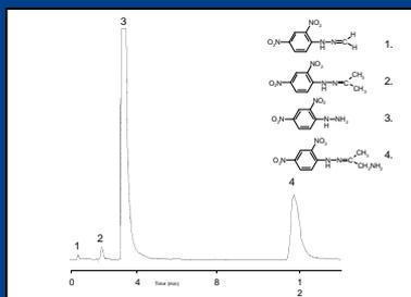
Fig. 2. HPLC chromatogram of a primary-treated effluent sample. For conditions see Material and Methods.
