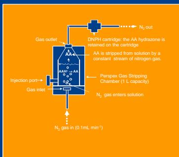
Fig. 1. Schematic representation of the gas stripping and derivatization system used for the determination of AA in aqueous samples
