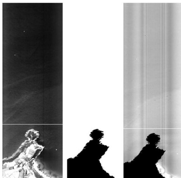
Figure 6. From left to right the images are of the uncorrected (490 nm waveband), non-water mask (black indicates the pixels that were masked) and atmospherically corrected (490 nm waveband) CASI imagery from the Rame Head end of the 10 000 feet Rame Head to Eddystone flightline. The imagery was flown at 11:55 on 9 August 1995 at a pixel resolution of approximately 6 m and heading of 19°. The white dot to the right of Rame Head (bottom of the image) and white line just above Rame Head indicate where the pixel (spectral values in figure 3) and swathe line (figure 4) were extracted from.
